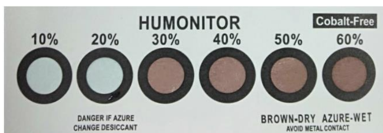
Figure 6. Humidity indicator card turns blue at 20%, baking is required
